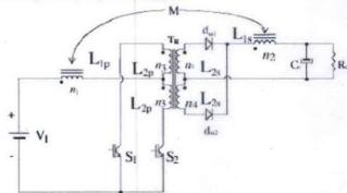
Fig 1 new flyback-current-fed push-pull dc-dc converter In order to miniaturize a converter it is preferred to use high switching frequency. Increasing the switching frequencies helps to reduce the volume of power supplies. In medium power applications where isolation is required, which can be achieved by transformers, fly-back [6] and forward converters [7].
