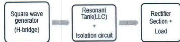
Fig. 3. Block diagram of LLC resonant converter
